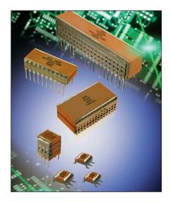
KYOCERA AVX is the original inventor of large capacitance value, stacked MLCC capacitors constructed with DIP leads. The SM-style, Switch Mode Power Supply (SMPS) capacitors were introduced by KYOCERA AVX in 1980s. These capacitors are the closest to the ideal electrical energy storage devices due to high CV product and extremely low ESR and ESL.
