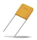
Automotive grade, AEC-Q200 qualified SV-style capacitors are designed with COG (NPO), class I dielectric that is characterized with very low dielectric losses. This product is designed for AC applications requiring capacitors capable of handling high AC currents at high frequencies.
